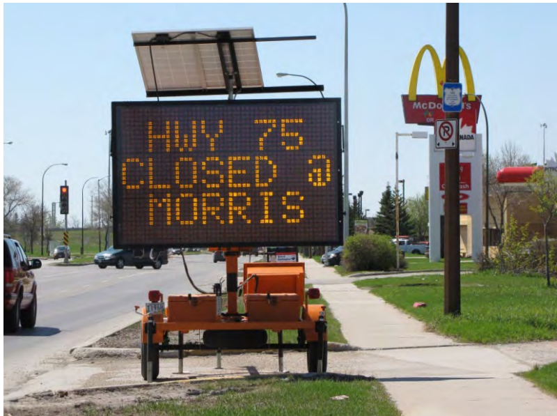
Figure 4.20: Alternative routing information displayed on a variable message sign
