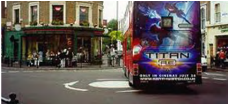
Figure 4.15: Vehicle driving over centre island of mini roundabout
