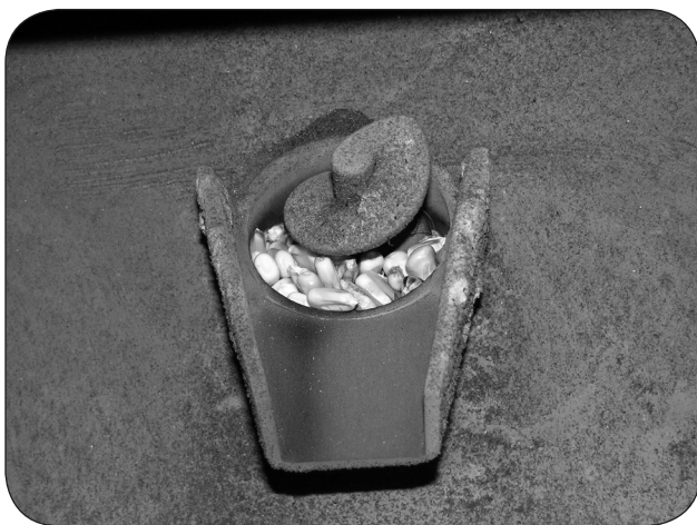
Figure 5. A fuel delivery auger as seen from inside the stove. The speed and operation are controlled by the stove control system. The shelled corn falls from the funnel below the auger discharge into the combustion chamber.
