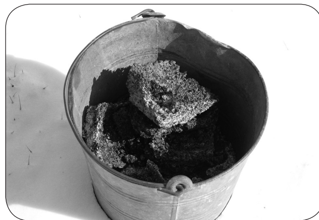
Figure 6. Store clinkers in a metal pail kept on a fireproof surface.
