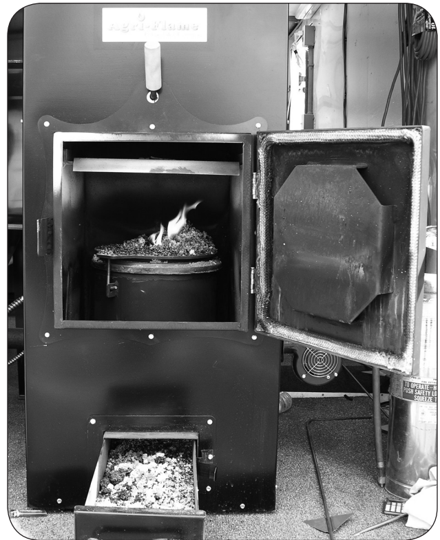
Figure 8. This corn burner uses a bottom fuel delivery system. Burnt corn can be seen mushrooming up and eventually falls into an ash tray.
