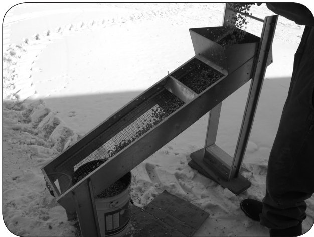
Figure 4. This home-built inclined screen is used to remove reddog and fines from shelled corn before it is burned. Do this job outside to prevent dust problems inside the house.
