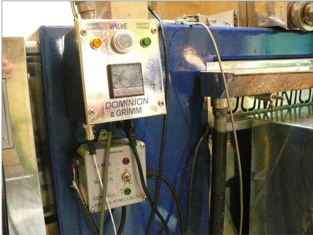
Figure 11. Control box/alarm connected to the sensor shuts down power to the oil burner if sap level gets too low in the pans.
