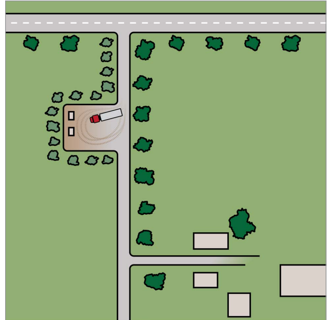
Figure 1. This drawing shows a storage/pick-up area for deadstock. Note that the site is out of public view.
