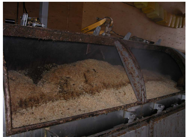
Figure 5. In-vessel composting system.
