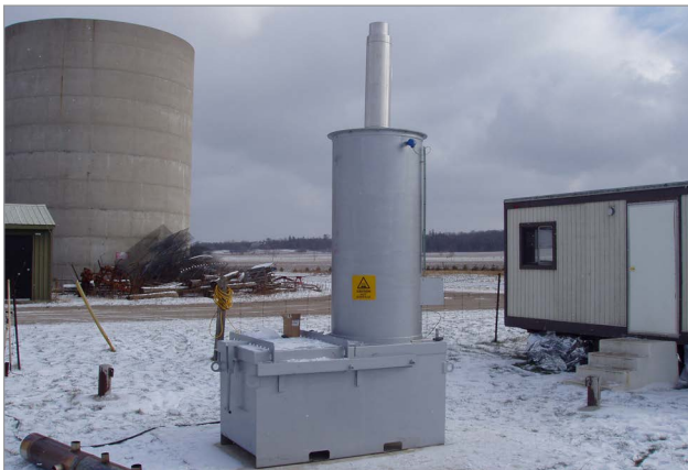
Figure 6. Incinerator with a secondary chamber.
