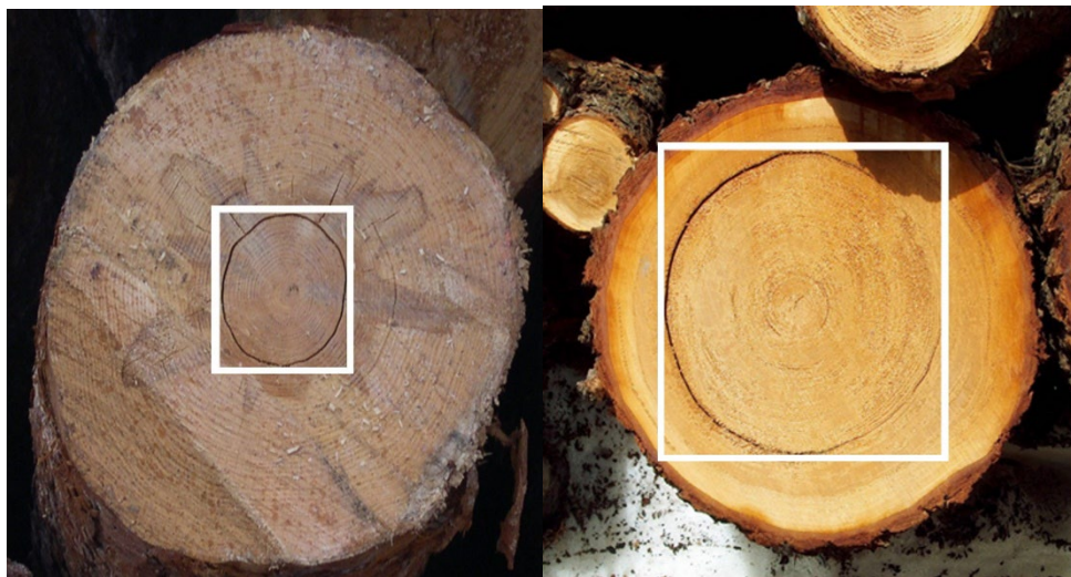
Figure 8 - Examples of shake
