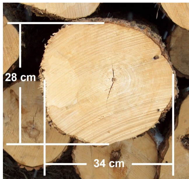
Figure 2 - Measuring diameters: logs with irregular sawn surfaces
