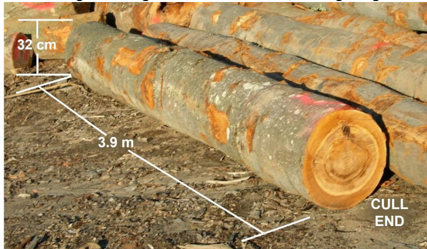
Figure 34 - A grade 2 beech log containing a defect
