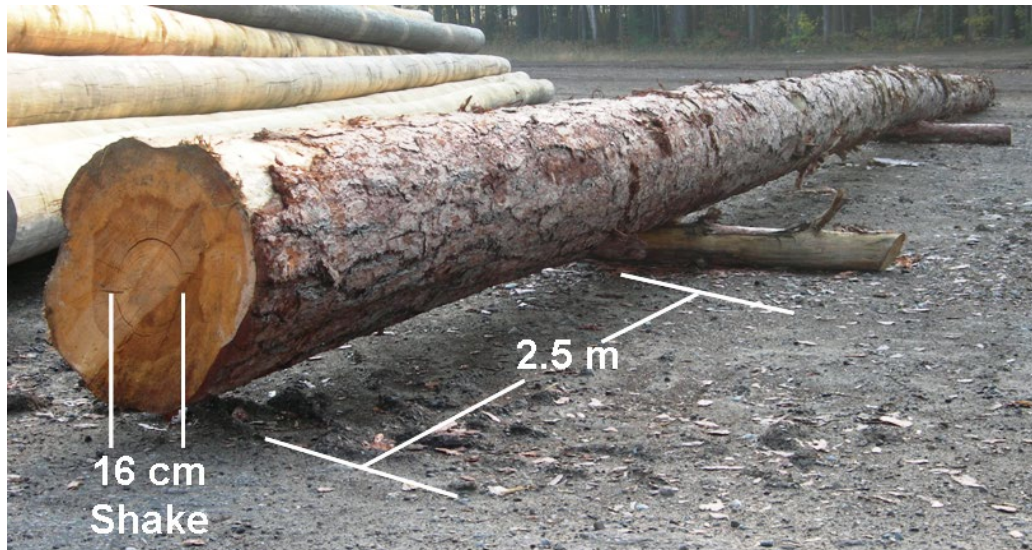
Figure 18 - Example of long timber with defect affecting one end only
