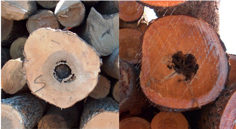
Figure 5 - Examples of heart rot
