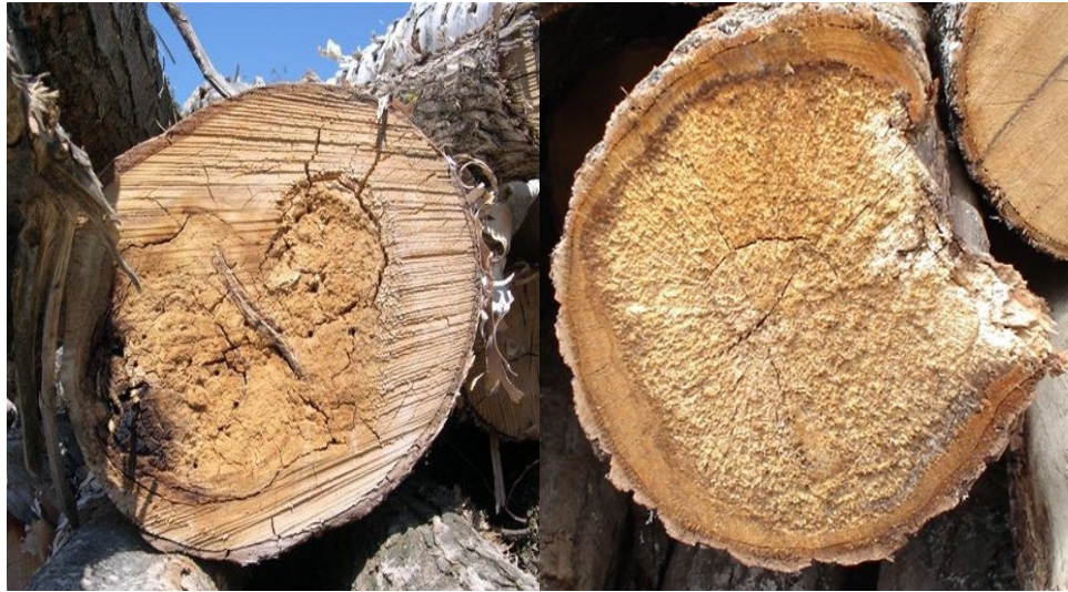
Figure 9 - Examples of punk rot
