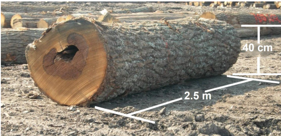
Figure 33 - A grade 1 oak log containing a partial defect
