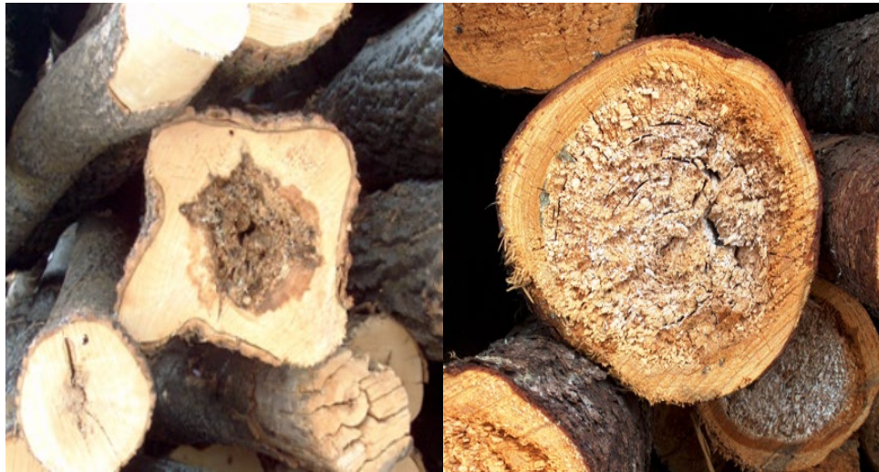
Figure 6 - Examples of stump rot
