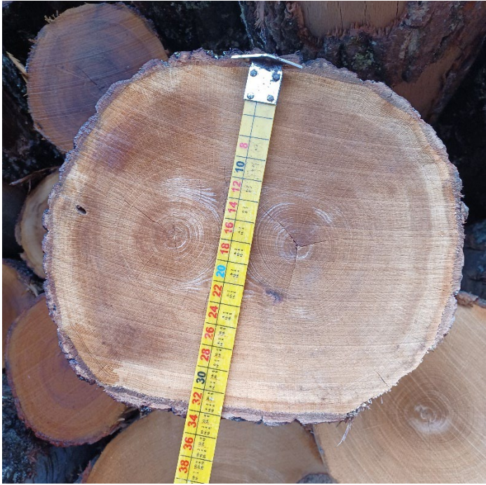
Figure 3 - Measuring diameters when cat's eyes are encountered
