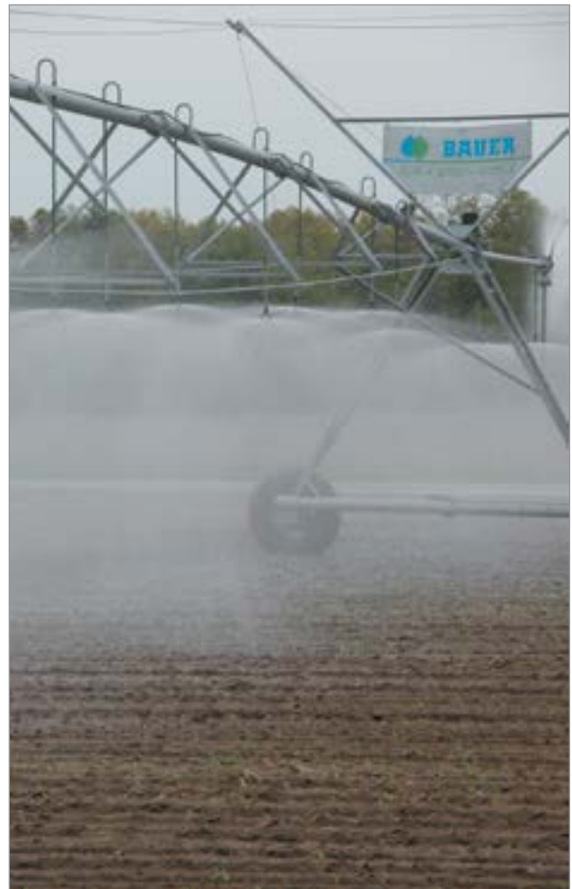
Figure 1. Low-pressure lateral-move irrigation system.
