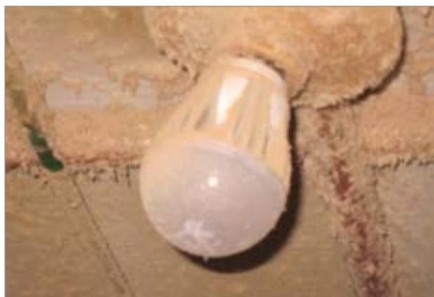
**Figure 7.** Edison-style LED bulb with heat dissipating fins covered in a layer of insulating dust. Source: National Poultry Technology Center, Auburn University, [www.poultryhouse.com](http://www.poultryhouse.com).
