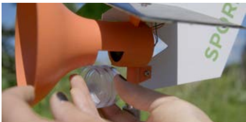
A Spornado cassette being removed from the device
