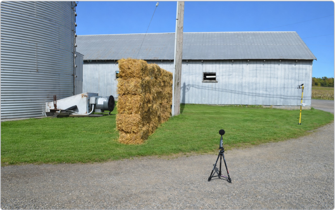
Figure 6. Grain bin axial aeration fan with a straw bale barrier placed at 4.35 m (14 ft) reduced the noise by 10 to 12 dB [5] in the region immediately behind the bale wall.
